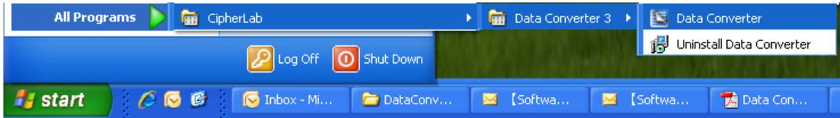
Data Converter is a long-running application known as Windows service that can be run in the background. You can find its icon in the bottom-right corner of the screen as the picture shown below.
