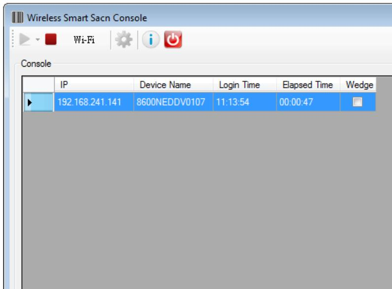
For Bluetooth connection, the Console area displays device name, login time, and elapsed time for each connected mobile computer or scanner.
