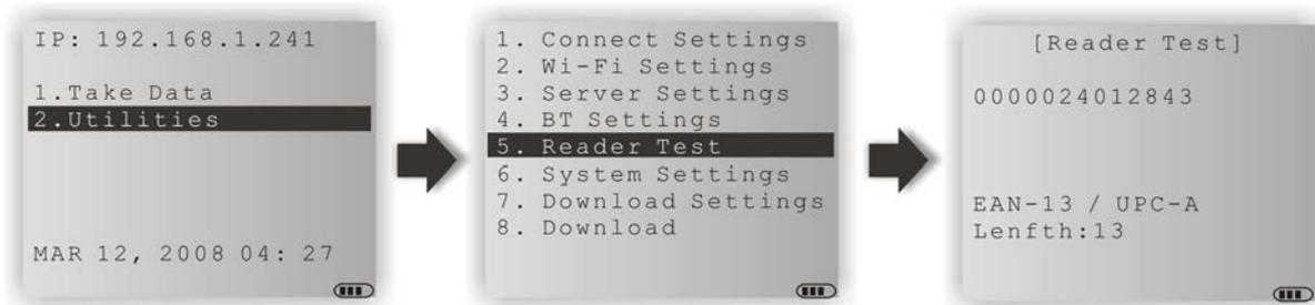
As the pictures illustrated above, users can press the trigger to scan barcode labels to make sure the barcode reader is working and identify the barcode type.
